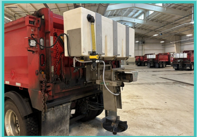
This Town of Canandaigua truck pre-wets salt before spreading, reducing bounce, scatter, and improving effectiveness. photo courtesy Canandaigua Lake Watershed Council
